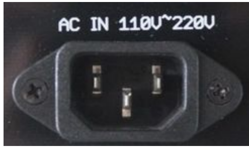
Picture 19 – 220V AC Input (UniPing server solution v3 device)
