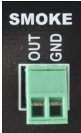
Picture 6 – Terminals «Smoke» (UniPing server solution v3 device)
