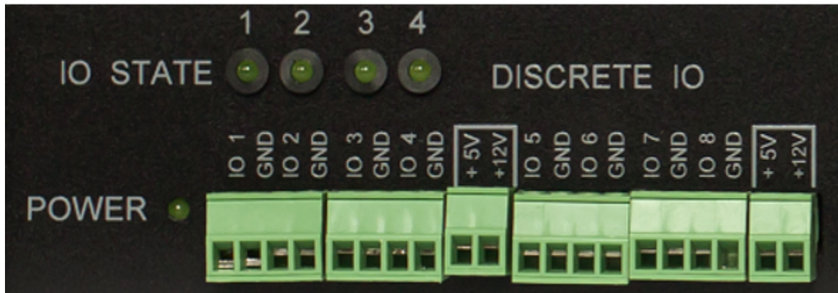
Picture 1 – A terminal block for connecting IO lines (UniPing server solution v3/SMS device)
