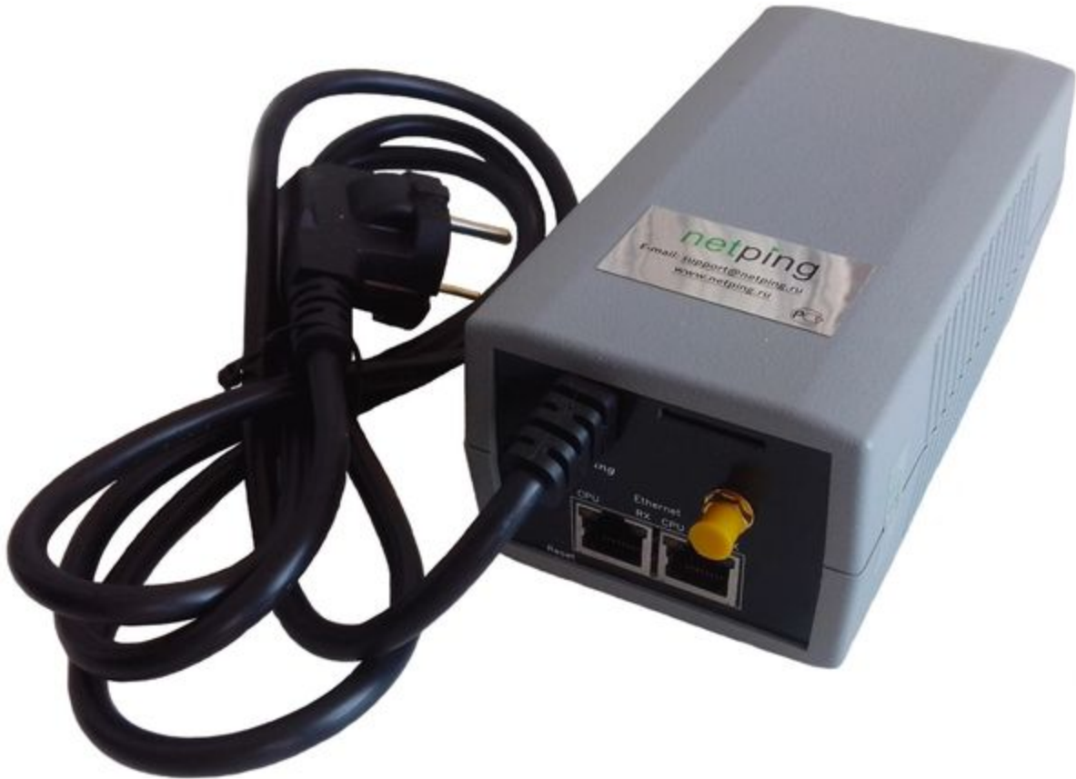
Picture 2 – Front view (NetPing 2/PWR-220 v2/SMS device)
